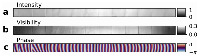
Fig. 6. Performance evaluation of the Talbot-Lau interferometer during rotation. a , the intensity has a characteristic maximum in the center and decreases to the left and right due to partial shadowing in the G_0 . b , the system visibility is highest in the center exceeding 26%, but due to partial shadowing there is a drop to the left and right. c , the interferometer phase is optimized for about 10 pixels per fringe for ideal phase sampling during processing and reconstruction.
