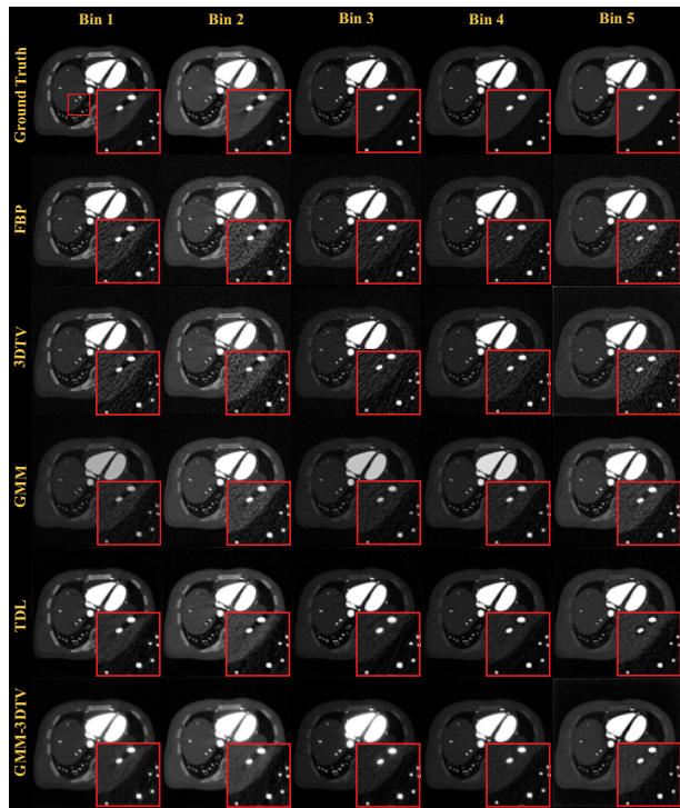
Fig. 2. Reconstructed images of the presented and compared methods on XCAT phantom. The display windows from Bin 1 to 5 are [0.00, 0.02] , [0.00, 0.010] , [0.00, 0.017] , [0.00, 0.015] and [0.00, 0.010] \text{mm}^{-1} , respectively. Zoomed ROIs indicated by the red box are displayed for better visualization.
