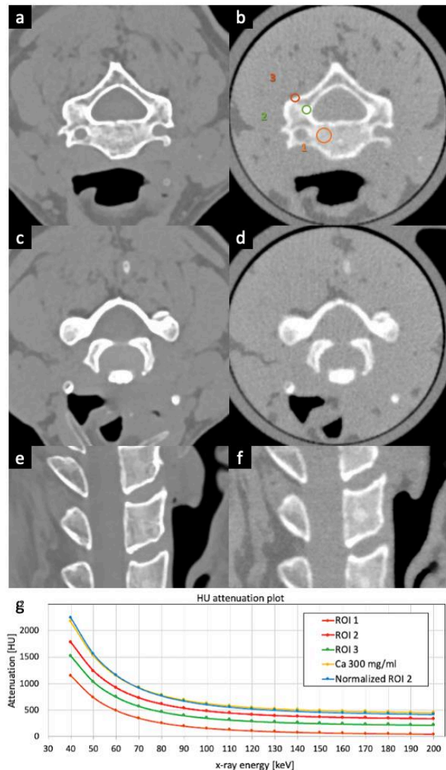
Fig. 3. Patient image and the PixelPrint cervical phantom. (a) (c) and (e) Original CT images utilized by PixelPrint to create the cervical phantom. (b) (d) and (f) CT images of the cervical phantom. All images have window level of 0 HU and width of 1200 HU. (g) Virtual monoenergetic HU measured with spectral CT at the denoted ROIs in (b) alongside reference values from a 300 mg/ml calcium insert (marked in yellow).
