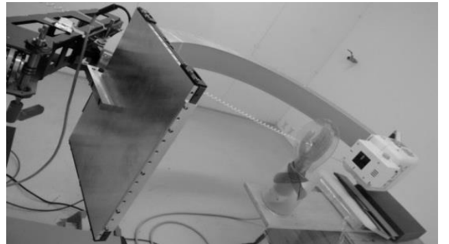
Fig. 3. Anthropomorphic hand phantom acquisition with an in-house C-arm device.
