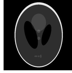
Fig. 1. The Shepp-Logan phantom, window: [-1000, 3400] HU.
