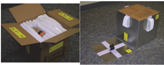
Figure 4. Photographs of a test data box with flannel fill, with and without the aluminum casing.
