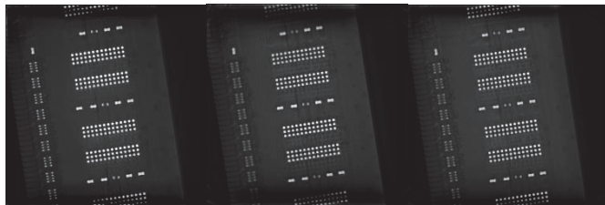
Fig. 4: In-plane slice image through reconstructed image. (from left to right) spherical sinusoidal, oblique tilted with 30 degree, and oblique tilted with 20 degree
