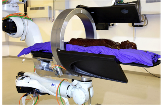
Fig. 1. Photography of a prototype of the Patient Alignment system with an Integrated x-ray imaging Ring (PAIR).
