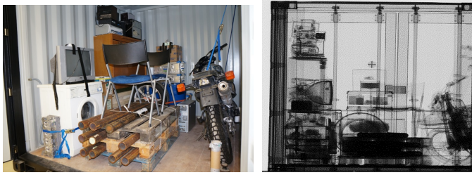
Fig. 4. Test container which was prepared with typical house moving cargo with a variety of different objects (left: photography, right: radiography).
