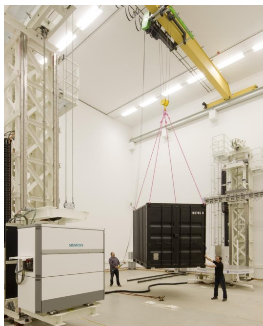
Fig. 1. The high-energy test facility is installed at the Fraunhofer EZRT, Fürth, Germany, and allows for reconstruction volumes of 3.2 meters in diameter and 5 meters in height.
