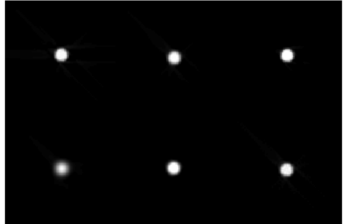
Fig. 3. Midplane reconstructions corresponding to various implementations of the directional derivative filter. The associated derivative filters are as follows: top row (from left to right): forward differencing, symmetric differencing, and linear (analogous to ramp filter); bottom row (from left to right): Hanning window of cutoff \frac{1}{2\Delta x} , Hanning window of cutoff \frac{1}{\Delta x} , and Hanning window of cutoff \frac{2}{\Delta x} . Note that the only obvious difference among any of the implementations is the blurring achieved by the low frequency cutoff Hanning filter.
