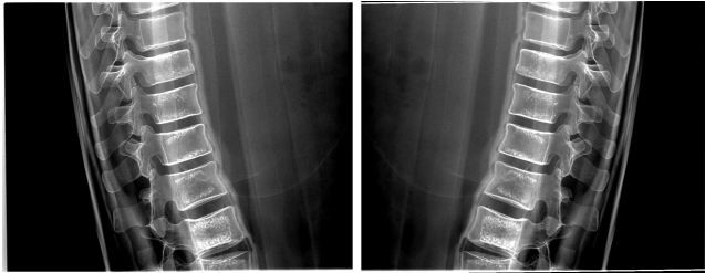
Fig. 8. The 50th rebinned projection of the torso phantom from the first sweep. Left: preprocessed; right: rebinned.
