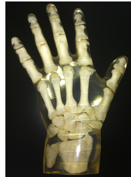
Figure 9. Hand phantom composed of bone encased in Lucite.
