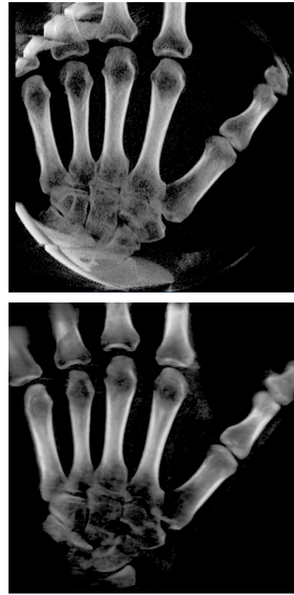
Figure 11. Volume view of hand phantom: (top) Reconstruction with distortion correction, (bottom) Reconstruction done by on-board system (Voxel size: (0.49\text{mm})^3 )
