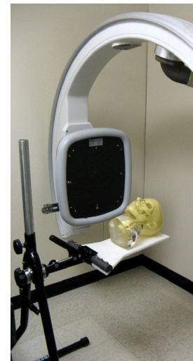
Fig. 5: FPD-based C-arm prototype, support stand, and anthropomorphic head phantom [4].
