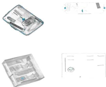
Fig. 5: Reconstruction examples of two bags. (Top) a mockup passenger bag, (Top Left) a 3-d volume rendering of the reconstruction (Top right) a transverse slice (Bottom) a mockup bag containing many sheet-like geometries. (Bottom left) a 3-d volume rendering of the reconstruction (Bottom right) a coronal slice through multiple of the slices, including a speaker cone. Note that image quality may have been intentionally degraded in these MV3D images.
