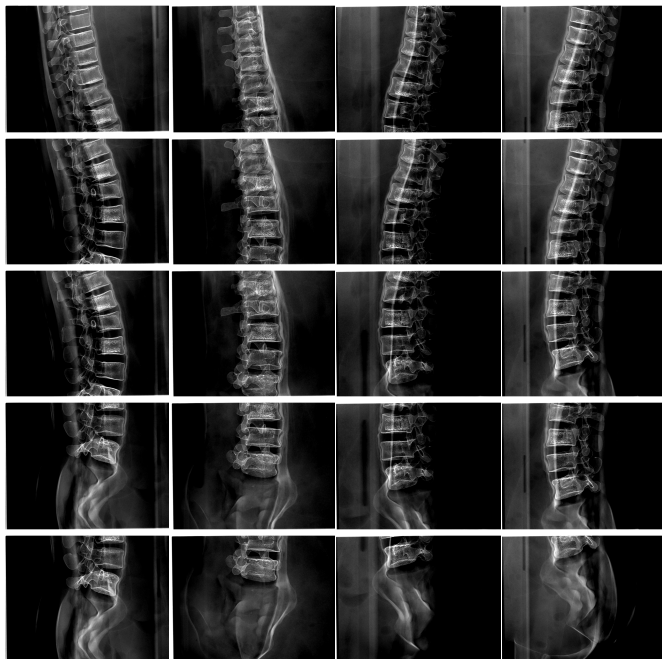
Fig. 2. Illustration of the preprocessed projections of the torso phantom. Top to bottom: 1st to 5th turn. Polar angle from left to right: 0^\circ , -80^\circ , -160^\circ and -230^\circ .
